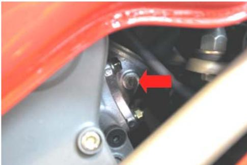
The RMV can be mounted visibly on the frame, or hidden behind the rear fairing. The more vertical the RMV the better and remember to avoid engine and exhaust components. For other fitting options see our easy step installation guide- '**RMV Positions, General**'.
